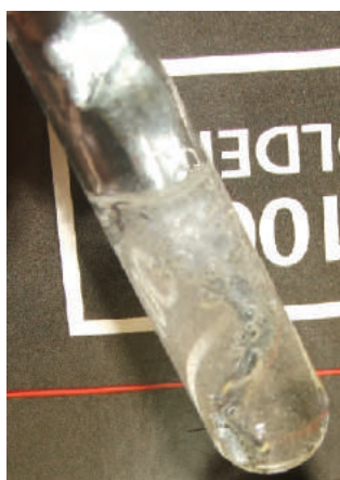
Figure 18.7 Zinc is an active transition metal. It dissolves in hydrochloric acid, forming a solution of colorless \text{Zn}^{2+} ions, \text{Cl}^- ions, and hydrogen gas.
