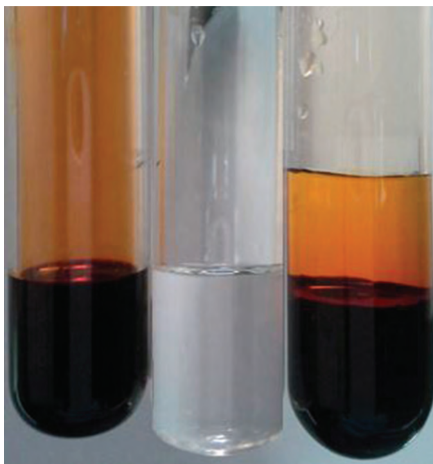
Figure 11.16 Bromine (the deep orange liquid on the left) and water (the clear liquid in the middle) are partially miscible. The top layer in the mixture on the right is a saturated solution of bromine in water; the bottom layer is a saturated solution of water in bromine. (credit: Paul Flowers)
