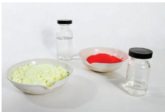
Figure 3.6 Each sample contains 6.02 \times 10^{23} molecules or formula units—1.00 mol of the compound or element. Clock-wise from the upper left: 130.2 g of \text{C}_8\text{H}_{17}\text{OH} (1-octanol, formula mass 130.2 amu), 454.9 g of \text{HgI}_2 (mercury(II) iodide, formula mass 459.9 amu), 32.0 g of \text{CH}_3\text{OH} (methanol, formula mass 32.0 amu) and 256.5 g of \text{S}_8 (sulfur, formula mass 256.6 amu). (credit: Sahar Atwa)
