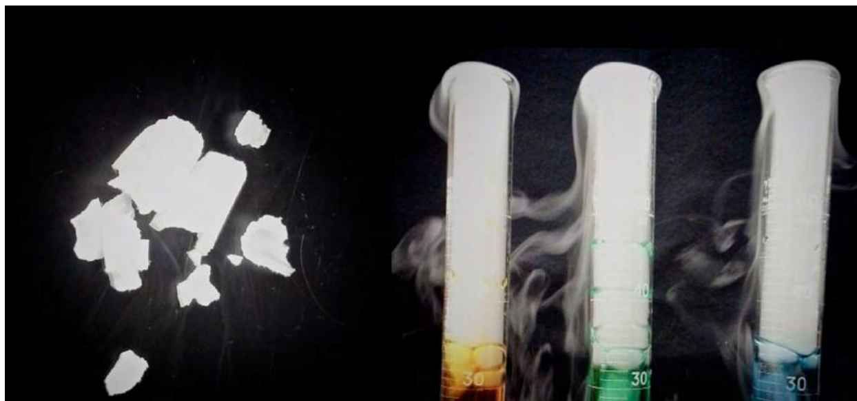
Figure 10.1 Solid carbon dioxide (“dry ice”, left) sublimates vigorously when placed in a liquid (right), cooling the liquid and generating a fog of condensed water vapor above the cylinder. (credit: modification of work by Paul Flowers)
