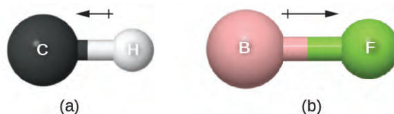
Figure 7.26 (a) There is a small difference in electronegativity between C and H, represented as a short vector. (b) The electronegativity difference between B and F is much larger, so the vector representing the bond moment is much longer.
