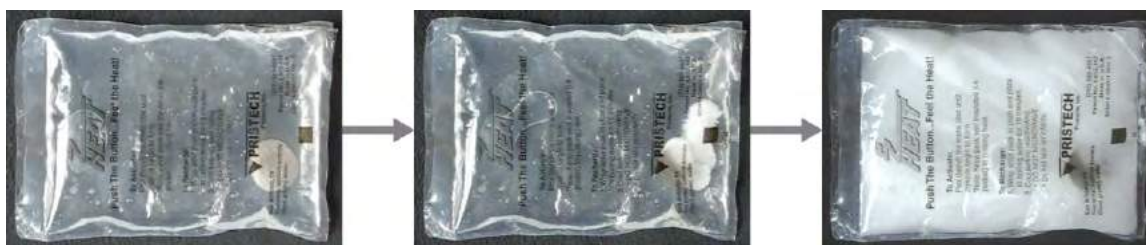
Figure 11.18 This hand warmer produces heat when the sodium acetate in a supersaturated solution precipitates. Precipitation of the solute is initiated by a mechanical shockwave generated when the flexible metal disk within the solution is “clicked.” (credit: modification of work by “Velela”/Wikimedia Commons)
