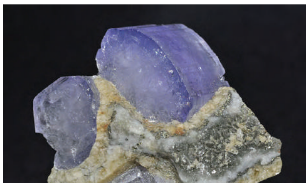
Figure 15.8 Crystal of the mineral hydroxylapatite, \text{Ca}_5(\text{PO}_4)_3\text{OH} , is shown here. Pure apatite is white, but like many other minerals, this sample is colored because of the presence of impurities.
