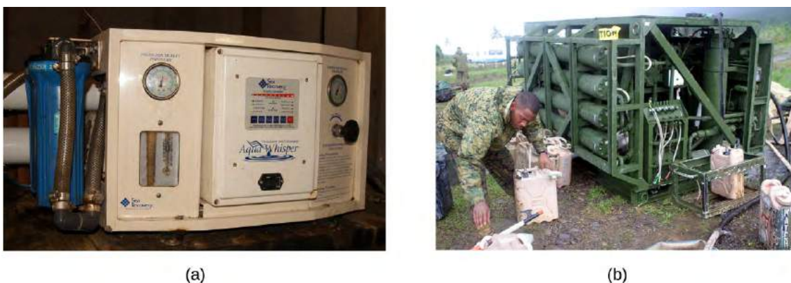
Figure 11.27 Reverse osmosis systems for purifying drinking water are shown here on (a) small and (b) large scales. (credit a: modification of work by Jerry Kirkhart; credit b: modification of work by Willard J. Lathrop)
