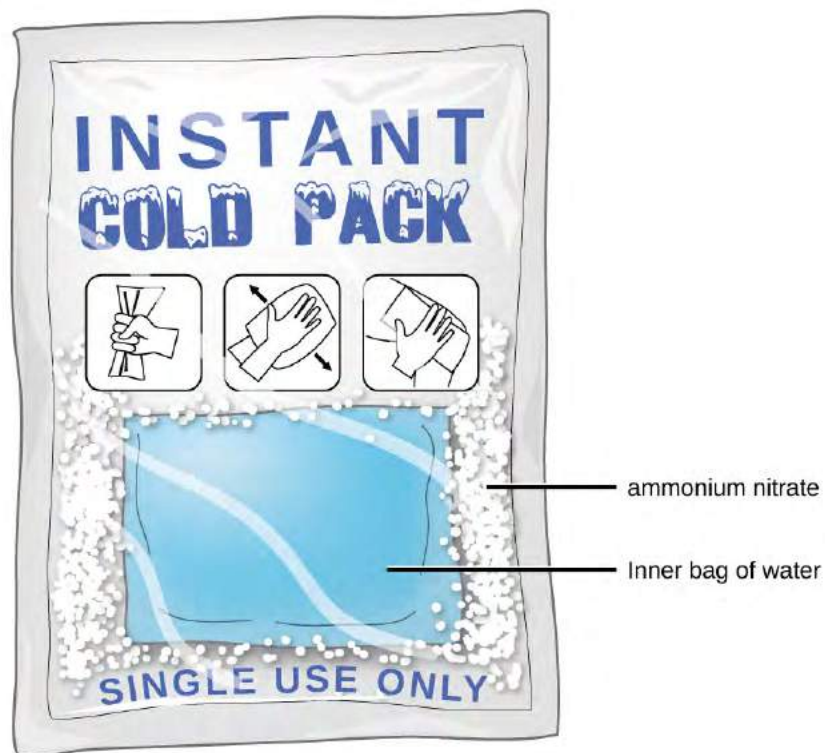
Figure 11.6 An instant cold pack gets cold when certain salts, such as ammonium nitrate, dissolve in water—an endothermic process.
