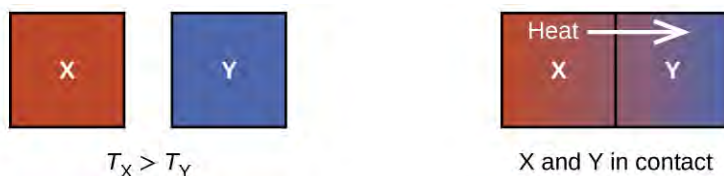
Figure 16.5 When two objects at different temperatures come in contact, heat spontaneously flows from the hotter to the colder object.
