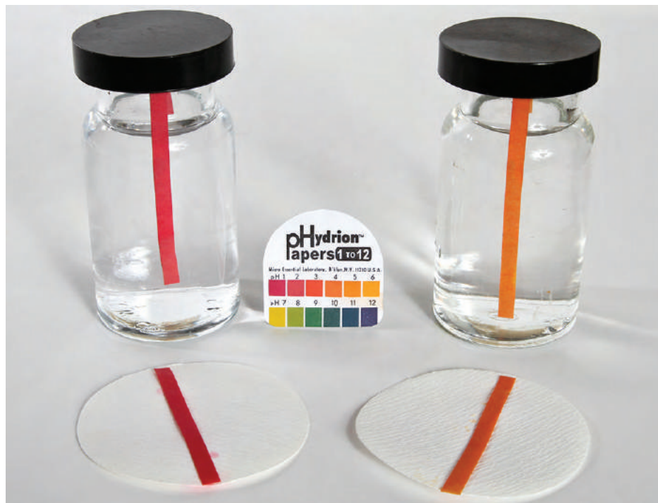
Figure 14.9 pH paper indicates that a 0.1- M solution of HCl (beaker on left) has a pH of 1. The acid is fully ionized and [\text{H}_3\text{O}^+] = 0.1\text{ M} . A 0.1- M solution of \text{CH}_3\text{CO}_2\text{H} (beaker on right) is has a pH of 3 ( [\text{H}_3\text{O}^+] = 0.001\text{ M} ) because the weak acid \text{CH}_3\text{CO}_2\text{H} is only partially ionized. In this solution, [\text{H}_3\text{O}^+] < [\text{CH}_3\text{CO}_2\text{H}] . (credit: modification of work by Sahar Atwa)
