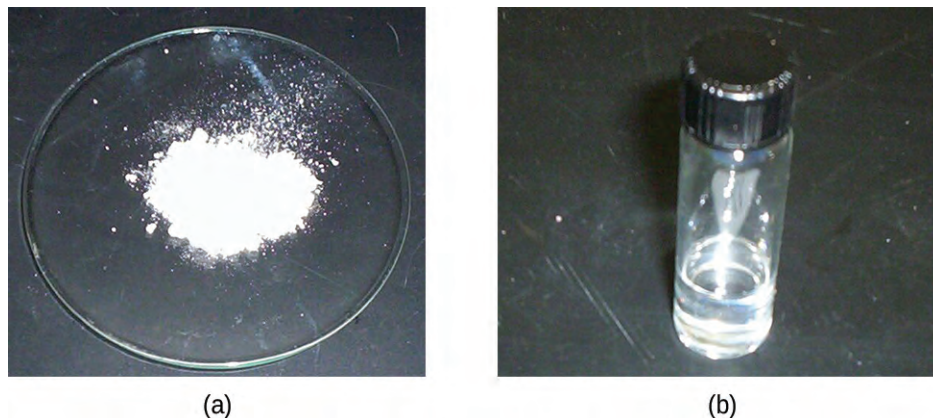
Figure 18.9 (a) Tin(II) chloride is an ionic solid; (b) tin(IV) chloride is a covalent liquid.
