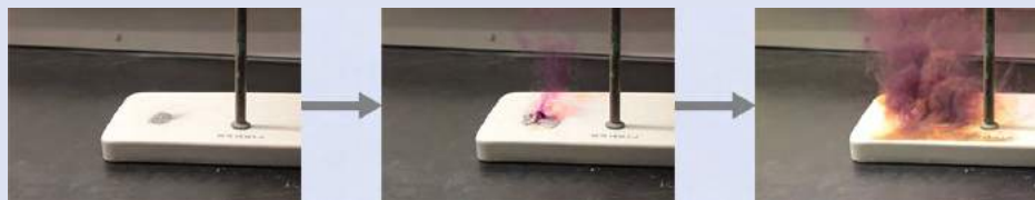
Figure 4.9 Aluminum and iodine react to produce aluminum iodide. The heat of the reaction vaporizes some of the solid iodine as a purple vapor. (credit: modification of work by Mark Ott)
