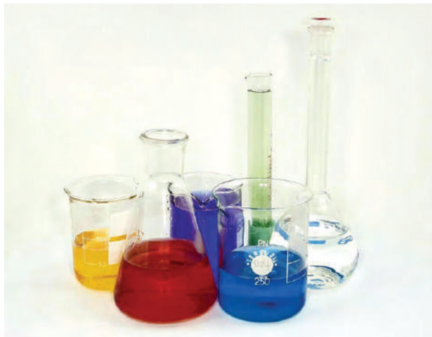
Figure 18.15 Laboratory glassware, such as Pyrex and Kimax, is made of borosilicate glass because it does not break when heated. The inclusion of borates in the glass helps to mediate the effects of thermal expansion and contraction. This reduces the likelihood of thermal shock, which causes silicate glass to crack upon rapid heating or cooling. (credit: "Tweenk"/Wikimedia Commons)
