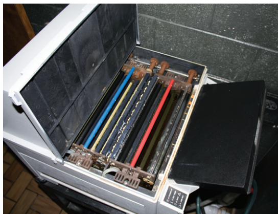
Figure 4.4. Automatic tabletop x-ray film processor crossover rollers.
