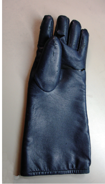
Figure 7.8. Lead glove with tear on palmar side of glove.
