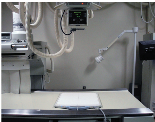
Figure 1.2. Canon DR panel tethered to be used tabletop or under table.
