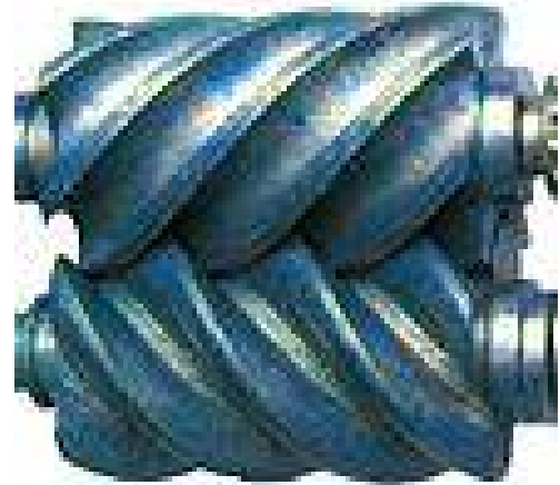
Lysholm screw compressor mechanism 295
