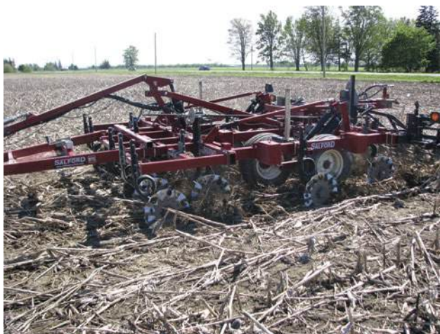
Photo 1–1. Vertical tillage tools are designed to manage and mix residue with light soil fractioning.
