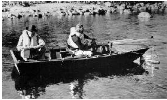
Figure 10-5 -- Making a current-meter measurement from a boat.
