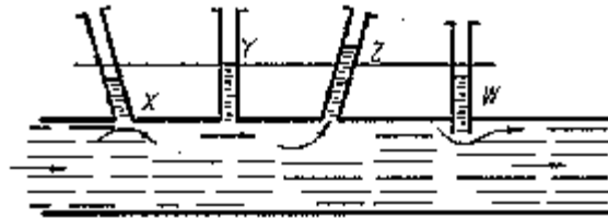
Figure 5-9 -- Examples of piezometer installation.
