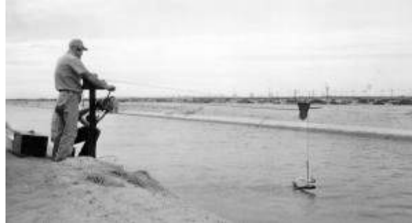
Figure 10-6 -- Cableway with traveling block to support the current meter and position it for readings. Counters are provided on the head tower and reel to determine the position of the meter in the channel.
