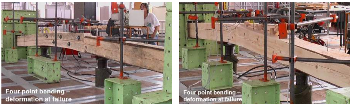
Figure 75 – Four point bending tests to compare the performance of steel and timber connections (ITAM, Prague).
