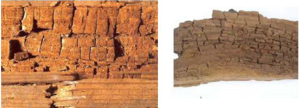
Figure 25 – Typical cube-like shapes of brown rot.
