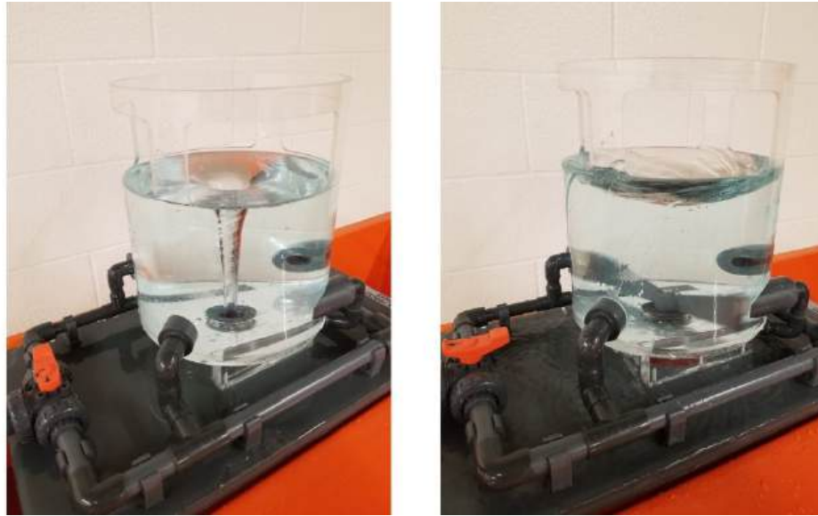
Figure 8.2: Free vortex (left) and forced vortex (right) produced in the lab
