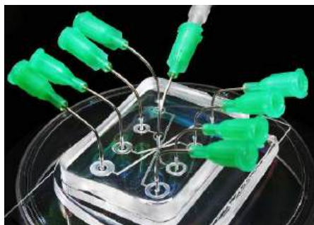
Figure (\PageIndex{11}): Lab-On-A-Chip Technologies. Example of a microfluidic lab-on-a-chip device sitting on a polystyrene dish. Stainless steel needles inserted into the device serve as access points for fluids into small channels within the device, which are about the size of a human hair. Image by National Institute of Standards and Technology (NIST)
