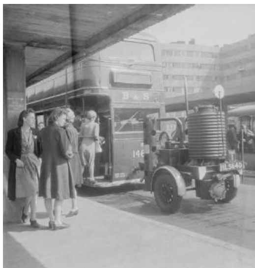
Figure 32.8.9: Bus power by wood gas c. 1943 in Leeds, England. By Ministry of Information Photo Division Photographer, Smith Norman? - http://media.iwm.org.uk/iwm/mediaLib.../large.jpg This is photograph D 15675 from the collections of the Imperial War Museums., Public Domain, https://commons.wikimedia.org/w/inde...curid=24364067
