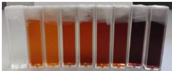
Figure 3.4.12: Example of a Chemical Reaction that causes a color change from orange to brown depending on increasing concentration. Image from: Ludwig, N., et. al. (2015) on Research Gate
