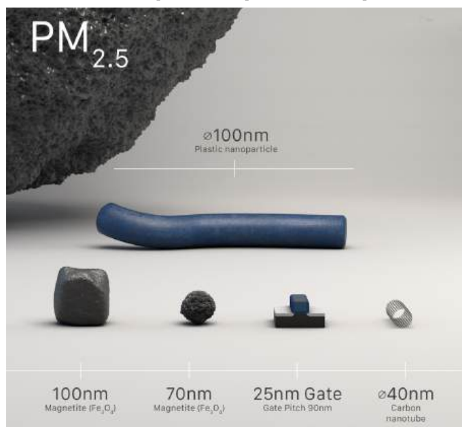
Figure 32.13.12: Relative sizes of PM0.1 particles compared to a PM2.5 particle. Sotirios Papathanasiou, ibid.
