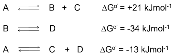
Figure 13.1.2: The Coupling of Two Reactions. The top reaction is nonspontaneous with a positive change in free energy of 21 kJ/mol. This reaction can be driven in the forward direction, by coupling it with a strongly spontaneous reaction that releases -34 kJ/mol. The overall net reaction has a negative change in free energy and is spontaneous
