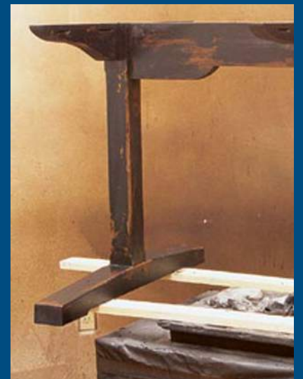
Here I've wiped the piece with a very wet cloth as the paint dried, which removed some of the paint, creating an antique finish.
