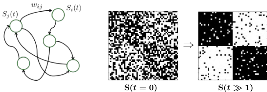
Figure 1.4: Recurrent neural networks. Left: A network of N = 5 neurons with partial connectivity and uni-directional synapses. Right: Pattern retrieval from a noisy initial configuration in a Hopfield network of 2500 units, storing 100 activity patterns. Activities S_j = \pm 1 are shown as black and white 'pixels', respectively. Initially, 40% of the S_j are flipped with respect to the pattern. The rightmost figure displays the system shortly before perfect retrieval is achieved.
