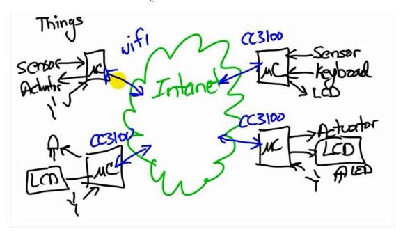
CC3100 is Wi-Fi and Internet-of-Things solution for MCU Applications. The CC3100 device is the industry's first Wi-Fi CERTIFIED chip used in the wireless networking solution. It is pin compatible with TM4C123GXL ARM Launchpad.
