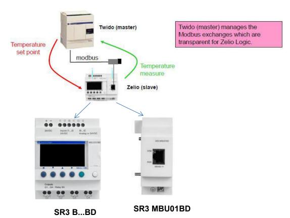
The temperature is measured by L35 high accuracy temperature sensor. Using the input word J1XT1 to write the temperature set point and the output word O1XT1 to read the measurement.
