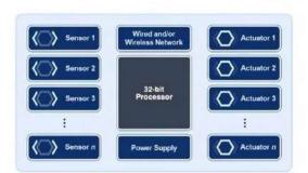
However, a common engineering compromise is to use two processors in the device. One low-cost processor is used for the physical-world interface, like a sensor. This would be an 8 or 16-bit chip. And a second 32-bit processor runs the network interface. This second processor is often placed in a separate module, one that can be certified separately for standards compliance.
