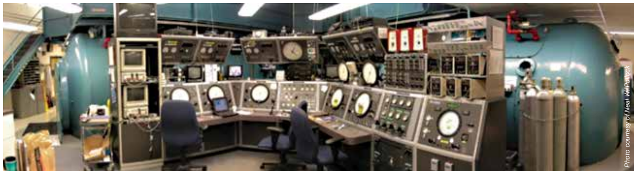
This is a large multiplace and multilock hyperbaric chamber, in which multiple pressure exposures can be conducted simultaneously.
