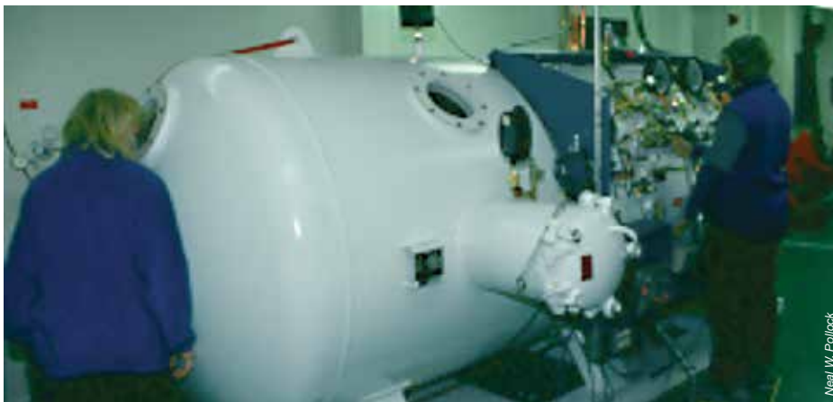
This is a small multiplace and multilock hyperbaric chamber; it can hold multiple patients plus inside tenders. Personnel or equipment can be transferred into or out of the chamber while treatment is ongoing.
