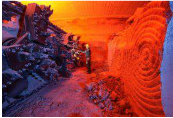
Figure 6.16 A mining machine at the face of potash ore (sylvite) in the Lanigan Mine near Saskatoon, Saskatchewan. The mineable potash layer is about 3 m thick.
