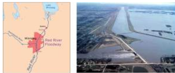
Figure 13.26 Map of the Red River Floodway around Winnipeg, Manitoba (left), and aerial view of the southern (inlet) end of the floodway (right). [Map from http://en.wikipedia.org/wiki/1997_Red_River_Flood#/media/File:Rednorthfloodwaymap.png and photo from Natural Resources Canada 2012, courtesy of the Geological Survey of Canada (Photo 2000-118 by G.R. Brooks).]
