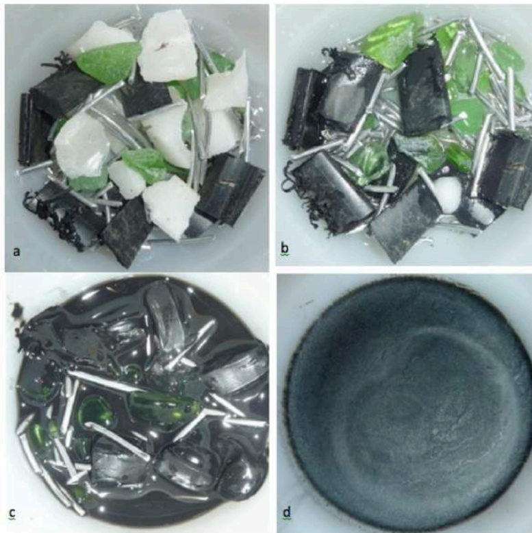
Figure 3.7 Partial melting of “pretend rock”: (a) the original components of white candle wax, black plastic pipe, green beach glass, and aluminum wire, (b) after heating to 50°C for 30 minutes only the wax has melted, (c) after heating to 120°C for 60 minutes much of the plastic has melted and the two liquids have mixed, (d) the liquid has been separated from the solids and allowed to cool to make a “pretend rock” with a different overall composition. [SE]
