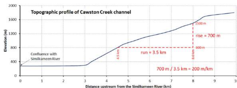
Figure 13.5 Profile of the main stem of Cawston Creek near Keremeos, B.C. The maximum elevation of the drainage basin is about 1,840 m, near Mount Kobau. The base level is 275 m, at the Similkameen River. As shown, the gradient of the stream can be determined by dividing the change in elevation between any two points (rise) by the distance between those two points (run). [SE]
