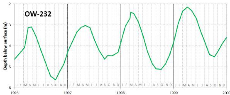
Figure 14.15 Water level data for B.C. observation well 232 for the period 1996 to 2000, showing seasonal variations [SE from data at: http://www.env.gov.bc.ca/wsd/data_searches/obswell/map/ ]
