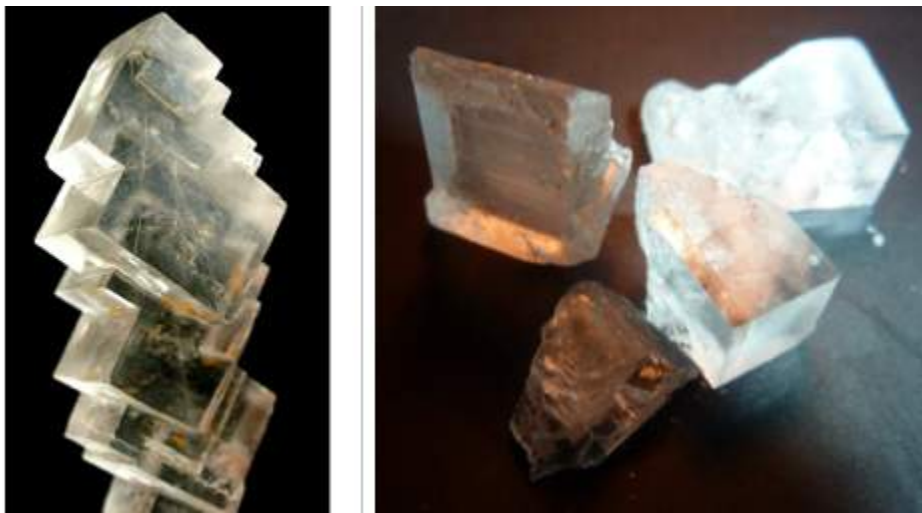
Figure 2.8 Cubic crystals (left) and right-angle cleavage planes (right) of the mineral halite. If you look closely at the cleavage fragment in the middle, you can see where it would break again (cleave) along a plane parallel to the existing surface.
