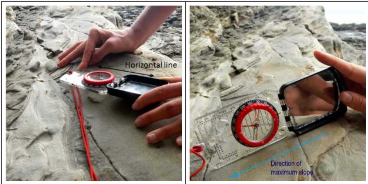
Figure 12.19 Measurement of strike (left) and dip (right) using a geological compass with a clinometer. [SE]
