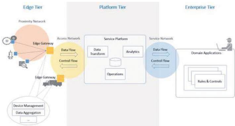
Figure 2-23. IIC implementation viewpoint reference architecture showing a three-tier network
