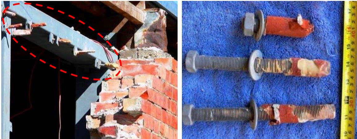
Figure C8.37: Failed adhesive brick anchors (Dizhur et al., 2013)
