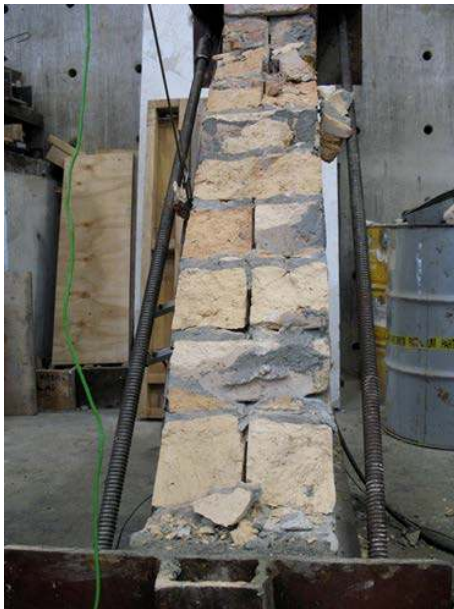
(b) Diagonal tension cracks to brick masonry. Note splitting of bricks, indicative of mortar stronger than bricks (Russell, 2010)
