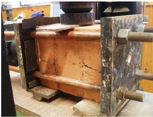
(a) Laboratory shear triplet test
