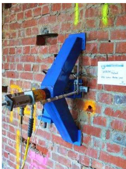
(a) Typical anchor pull test set-up
