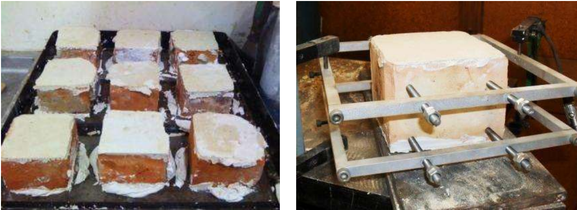
Figure C8A.5: Brick and mortar sample and compression test set-up (EQ STRUC Ltd)
