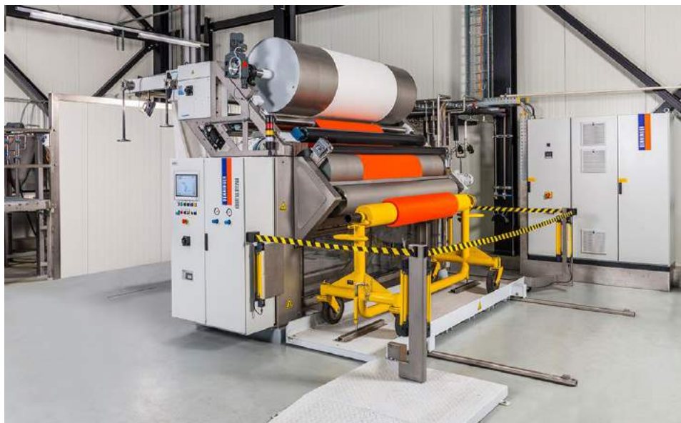
Figure 3-7: Cold pad batch (CPB) dyeing station [24, p. 13]
