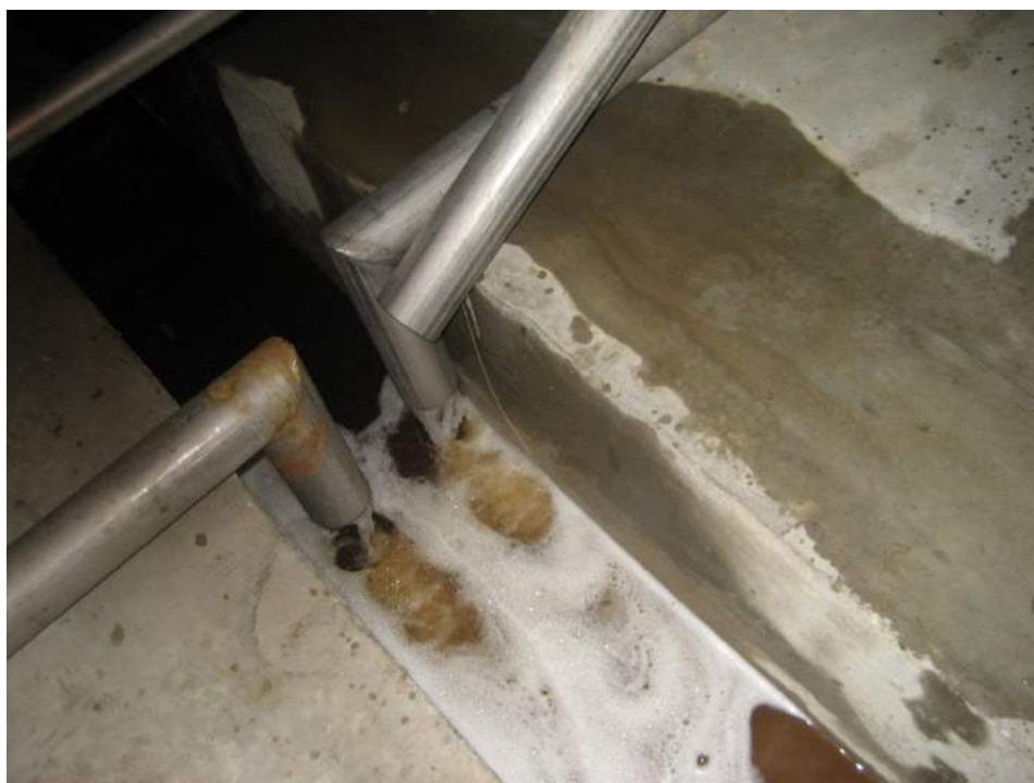
Figure 3-10: Chemical loss by uncontrolled liquor pick-up [22]
