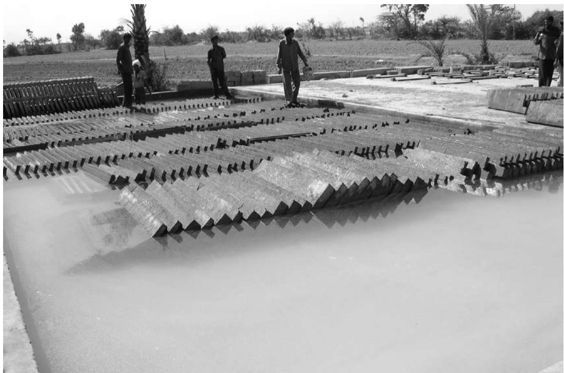
Water tank curing method. Cement products are only partly immersed into water, resulting into loss of quality
