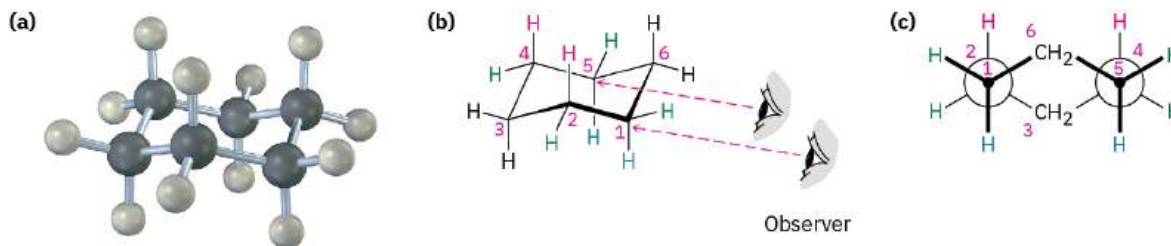
FIGURE 4.8 The strain-free chair conformation of cyclohexane. All C–C–C bond angles are 111.5^\circ , close to the ideal 109^\circ tetrahedral angle, and all neighboring C–H bonds are staggered.
