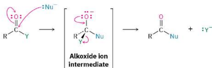
FIGURE 21.2 The general mechanisms of nucleophilic addition and nucleophilic acyl substitution reactions. Both reactions begin with addition of a nucleophile to a polar C=O bond to give a tetrahedral, alkoxide ion intermediate. (a) The intermediate formed from an aldehyde or ketone is protonated to give an alcohol, but (b) the intermediate formed from a carboxylic acid derivative expels a leaving group to give a new carbonyl compound.
