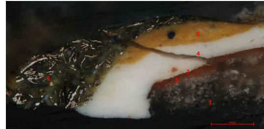
Figure 7. OM cross section from the stofato on the white dress.
