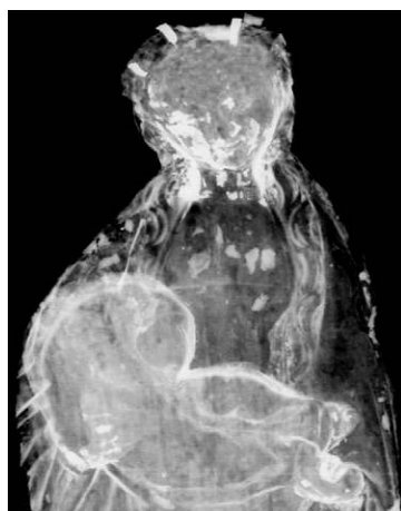
Figure 4. Detail of the X-radiograph showing the carved block of walnut tree. © Division of Photography and Radiography.
