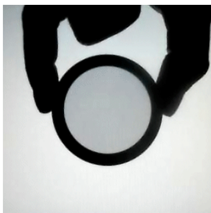
Figure 100 A polaroid filter allows light through only if the light is polarized at the same angle as the filter.
