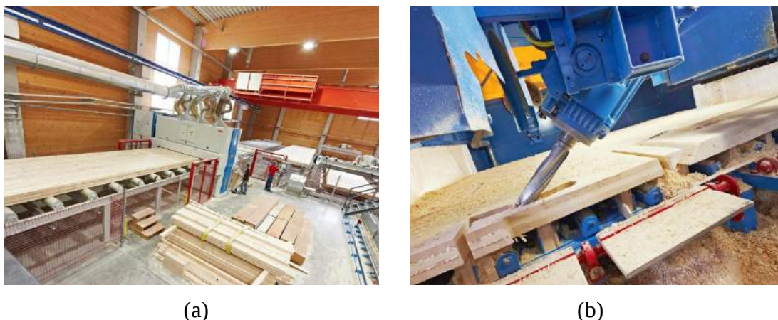
Figure 5 – Manufacturing of CLT; (a) Sanding of CLT surfaces; (b) CNC processing.
