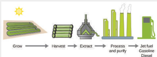
Figure 5. Algae convert sunlight and carbon dioxide into oil that is harvested, extracted, purified, and transformed into a variety of renewable fuels.
