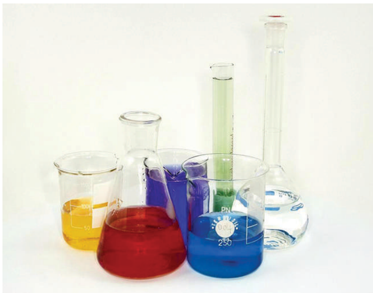
Figure 4. Laboratory glassware, such as Pyrex and Kimax, is made of borosilicate glass because it does not break when heated. The inclusion of borates in the glass helps to mediate the effects of thermal expansion and contraction. This reduces the likelihood of thermal shock, which causes silicate glass to crack upon rapid heating or cooling. (credit: “Tweenk”/Wikimedia Commons)
