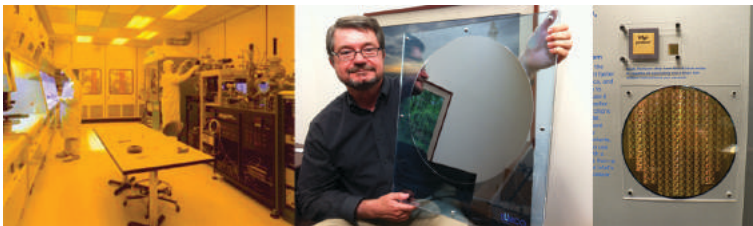
Figure 1. Purity is extremely important when preparing silicon wafers. Technicians in a cleanroom prepare silicon without impurities (left). The CEO of VLSI Research, Don Hutcheson, shows off a pure silicon wafer (center). A silicon wafer covered in Pentium chips is an enlarged version of the silicon wafers found in many electronics used today (right). (credit middle: modification of work by “Intel Free Press”/Flickr; credit right: modification of work by Naotake Murayama)
