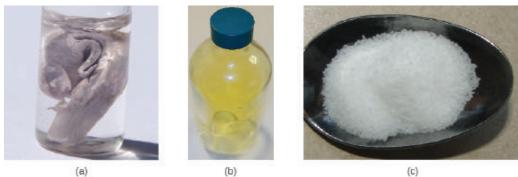
Figure 1. (a) Sodium is a soft metal that must be stored in mineral oil to prevent reaction with air or water. (b) Chlorine is a pale yellow-green gas. (c) When combined, they form white crystals of sodium chloride (table salt). (credit a: modification of work by “Jurii”/Wikimedia Commons)
