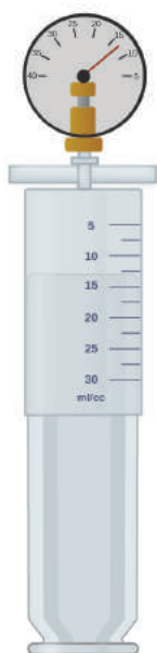
Figure 5. When a gas occupies a smaller volume, it exerts a higher pressure; when it occupies a larger volume, it exerts a lower pressure (assuming the amount of gas and the temperature do not change). Since P and V are inversely proportional, a graph of 1/P vs. V is linear.
