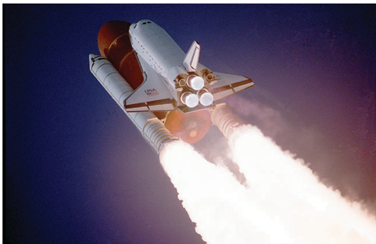
Figure 3. Before the fleet's retirement in 2011, liquid hydrogen and liquid oxygen were used in the three main engines of a space shuttle. Two compartments in the large tank held these liquids until the shuttle was launched. (credit: "reynermedia"/Flickr)
