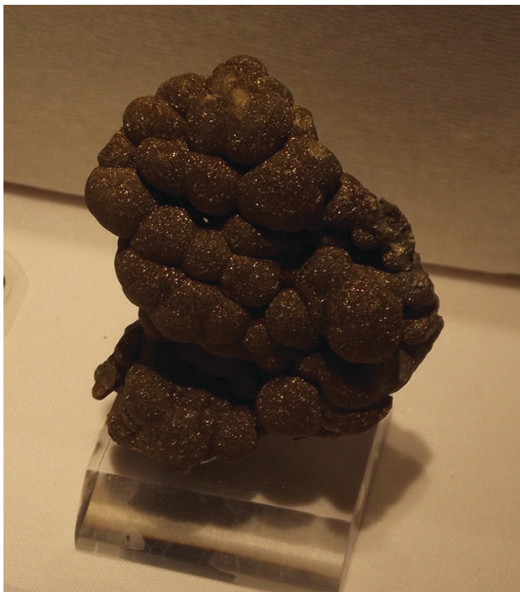
Figure 7. Blister copper is obtained during the conversion of copper-containing ore into pure copper. (credit: "Tortie tude"/Wikimedia Commons)
