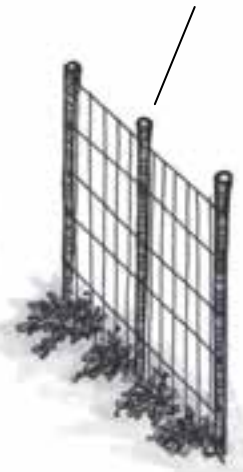
Chicken wire or hardware cloth supported by rebar
