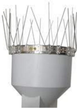
Figure 13.12: Bird protector for rain gauge (Source: Pacher).
