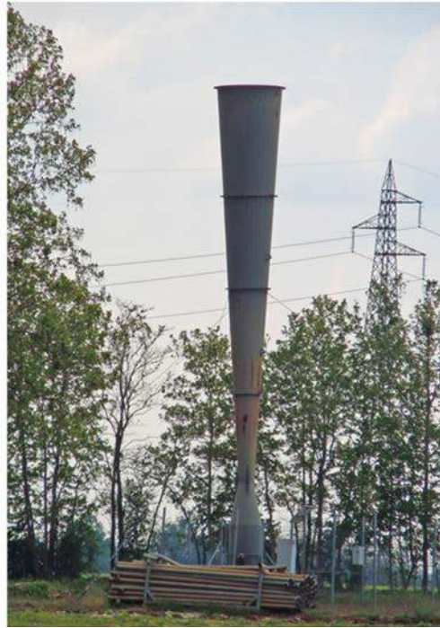
Figure 9.3: Hail cannon (Source: Massimo Telò – Own work, CC BY–SA 3.0, https://commons.wikimedia.org/w/index.php?curid=19250054 ).
