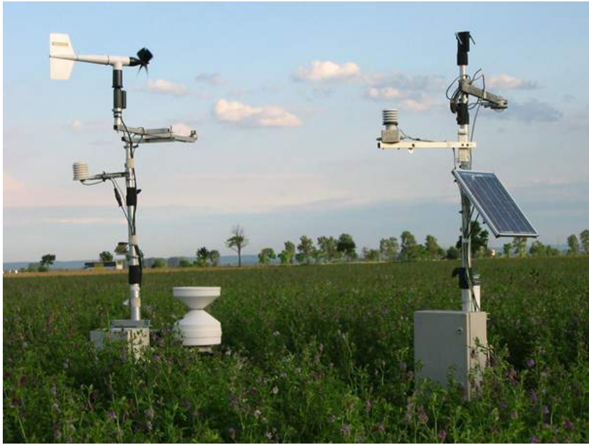
Figure 13.20: Agrometeorological weather stations (with variety of sensors) in an alfalfa field for crop water balance estimations (Source: BOKU–Met).
