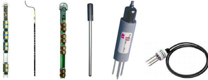
Figure 13.14: Various FDR/TDR soil moisture probes from different producers. From left to right: Sentek EnviroSmart, Delta-T Profile Probe, Agrilink C-Probe, AquaCheck, Delta-T Profile Probe and Stevens Hydra Probe, (Source: Pacher).
