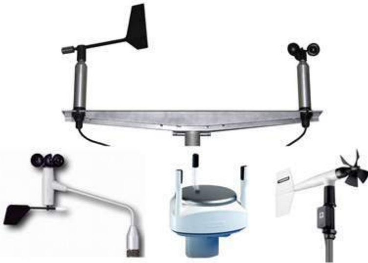
Figure 13.10: Various wind sensors, including propeller (bottom right), wind cap and ultra-sonic sensor (bottom center); (Source: Pacher).
