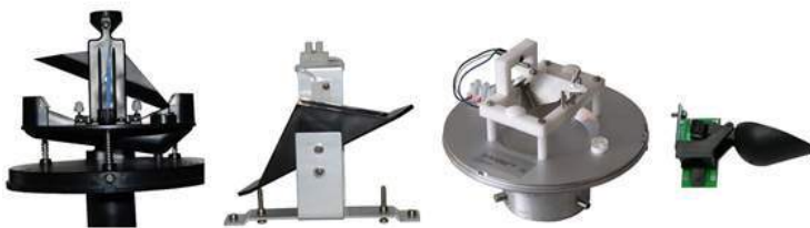
Figure 13.11: Various rain gauge (tipping bucket) mechanics (Source: Pacher).
