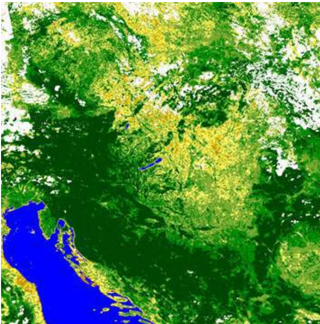
Figure 14.6: Atmospherically corrected NDVI map of Hungary. NOAA/AVHRR 10-day composite image of 1–10 September 1997 (Nejedlik and Orlandini, 2008).
