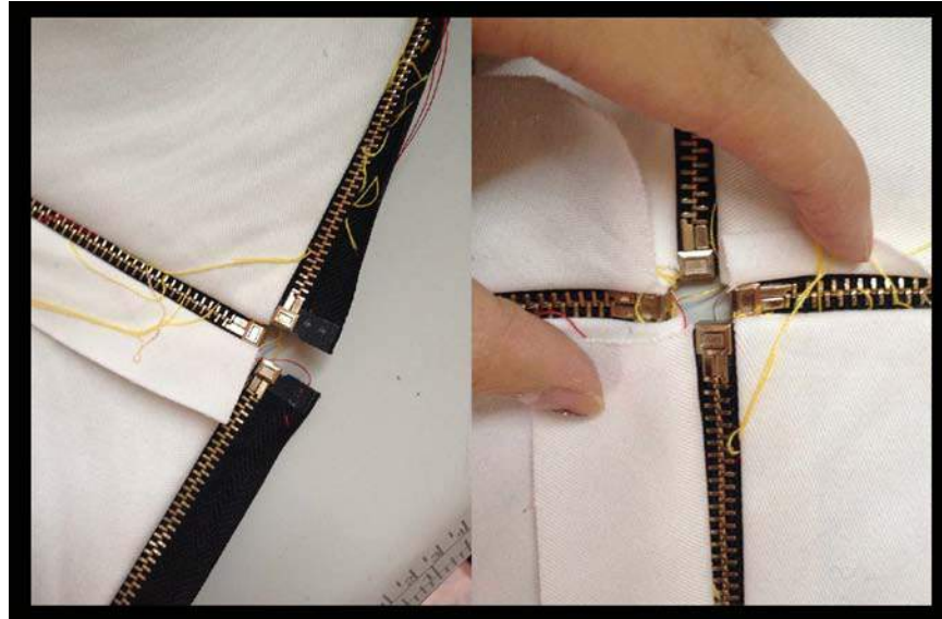
Figure 7.1. Sample making for zipper cross-connection technique
