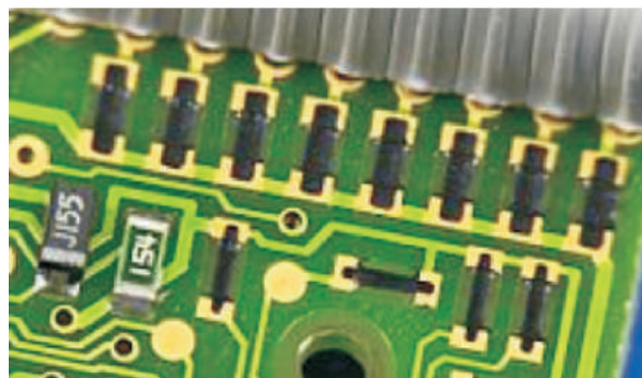
Figure-7 : A Carbon Resistor Printed Directly onto the SMD pads on a PCB
