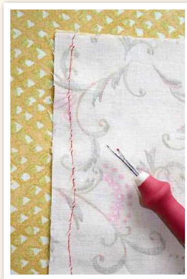
Use your seam ripper as shown to cut through every second or third stitch.
