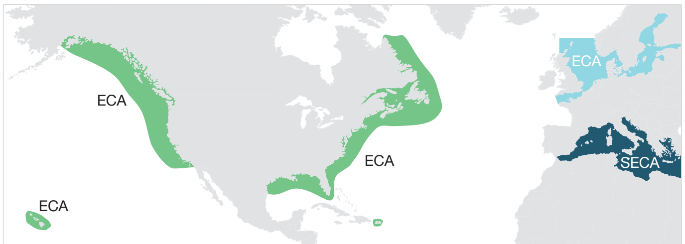
Fig. 4.05: Existing SO x & NO x emission control areas around North America and North Europe, and SO x emission control area in the Mediterranean
