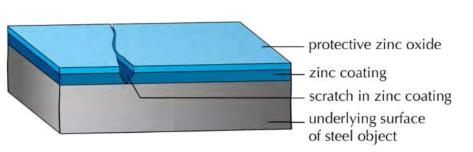
A segment of galvanised steel, showing damage to the zinc coating.
