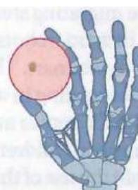
Biomimetic hand It mimics the human hand with artificial joint capsules and rubber ligaments and tendons.
