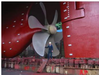
The white patches visible on the ship's hull are zinc block sacrificial anodes.
