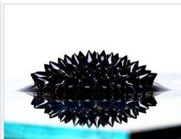
A ferrofluid containing superparamagnetic \text{Fe}_3\text{O}_4 nanoparticles, which are coated with oleic acid and suspended in oil, in the field of a strong permanent magnet.
