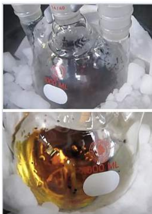
Solutions of lithium metal in liquid ammonia at low (top, ionic conductor) and higher (bottom, metal) Li concentration. From a video by Joshua Judkins
