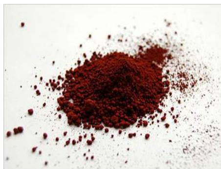
Fe 2 O 3 powder is reddish orange because of its 2.2 eV band gap
