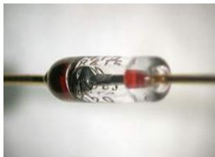
Closeup of a diode, showing the square-shaped semiconductor crystal ( black object on left ) (John Maushammer, Wikipedia , CC-BY-SA)
