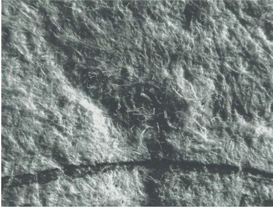
Figure A.9.d. Urs Graf, Two Landsquenets with a Maid and Death . Microphotograph of part of the false bull's head watermark, showing roughening and cutting of the paper fibers.
