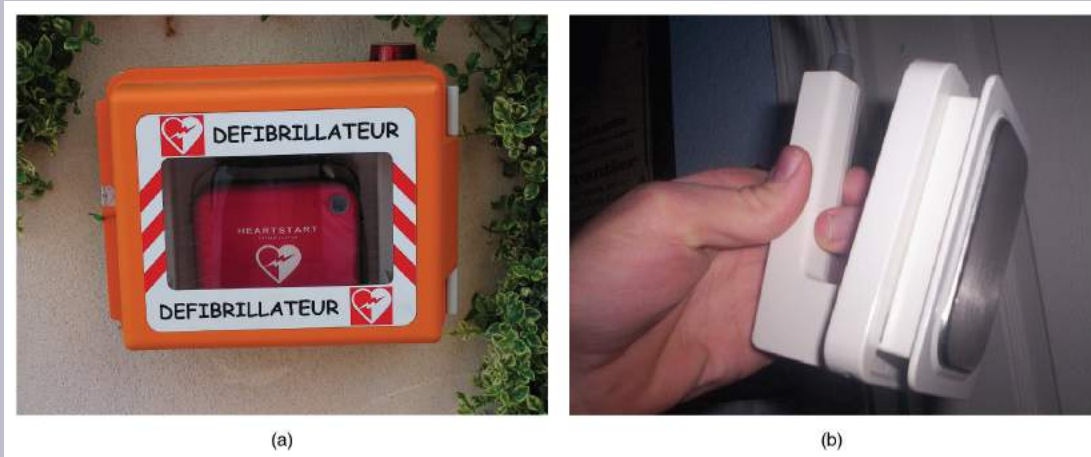
Figure 19.2.10 – Defibrillators: (a) An external automatic defibrillator can be used by nonmedical personnel to reestablish a normal sinus rhythm in a person with fibrillation. (b) Defibrillator paddles are more commonly used in hospital settings. (credit b: “widerider107”/flickr.com)
