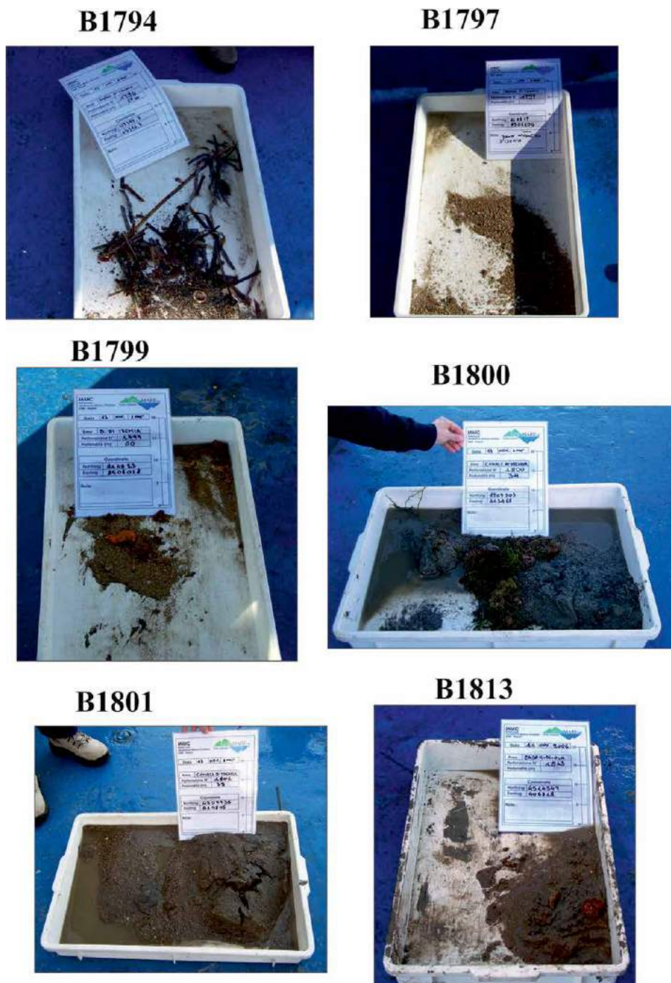
Figure 5. Sea bottom samples showing the occurrence of bioclastic deposits in the Ischia offshore.
