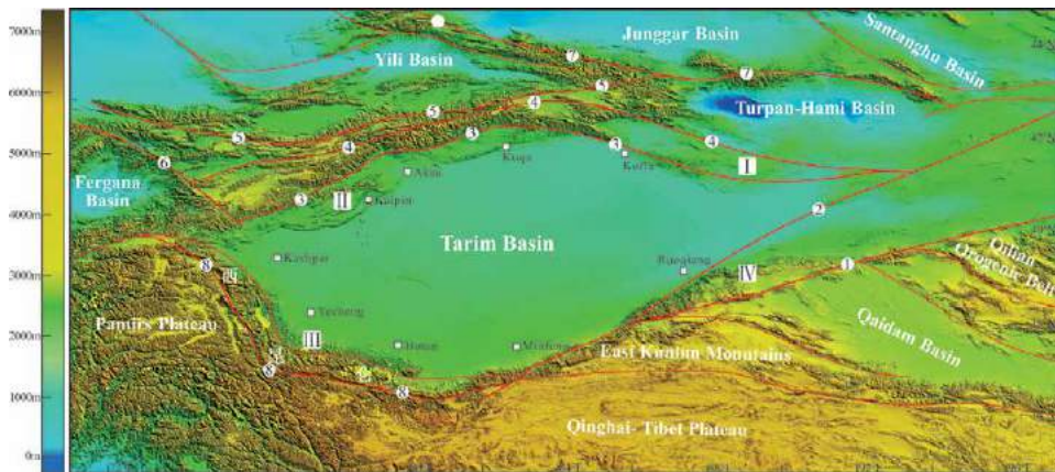
Figure 1. Tectonic characteristics of the Tarim Basin and its peripheral areas. I-Kuruktag Quruqtagh uplift belt; II-Kalpin uplift belt; III-Tiekelike uplift belt; and IV-Altun uplift belt. 1-Altun strike-slip fault; 2-Xingxingxia strike-slip fault; 3-North Tarim fault; 4-south marginal fault of the central Tianshan; 5-Nikolaev-Nalat fault belt; 6-Talass-Fergana strike-slip fault; 7-north Tianshan suture belt; and 8-Kangxiwar fault belt.
