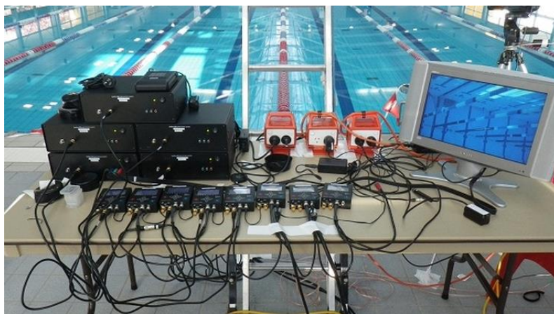
Fig.48: 3D body scanning, 17-camera biomechanical device
