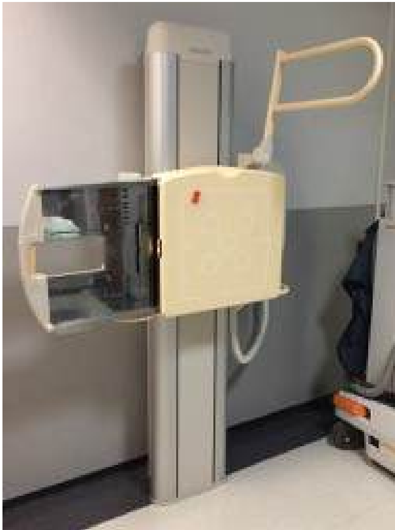
Figure 3.6A A standard, fixed location, wall, x-ray detector used for upright chest and abdomen x-rays
