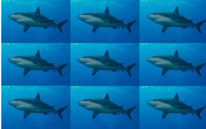
Figure G.4: The object plane as modeled by cyclic convolution and Fourier transforms. The multiple sharks (extending to \infty in all directions) illustrate the periodicity inherent in the use of cyclic convolution and Fourier transforms.
