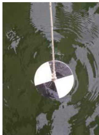
Figure 16.21: A black-and-white Secchi disk as used in limnology.
