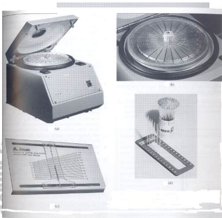
Fig. 10.2 (a) Microhematocrit centrifuge (b) Spiral reader located on the rotor head, used to read PCVs after centrifuging. (c) Graph PCV reader. (d) Sealant used to seal capillaries.
