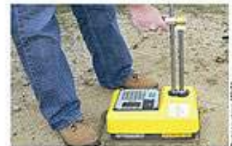
A moisture density gauge indicates whether a foundation is suitable for constructing a building or roadway.
