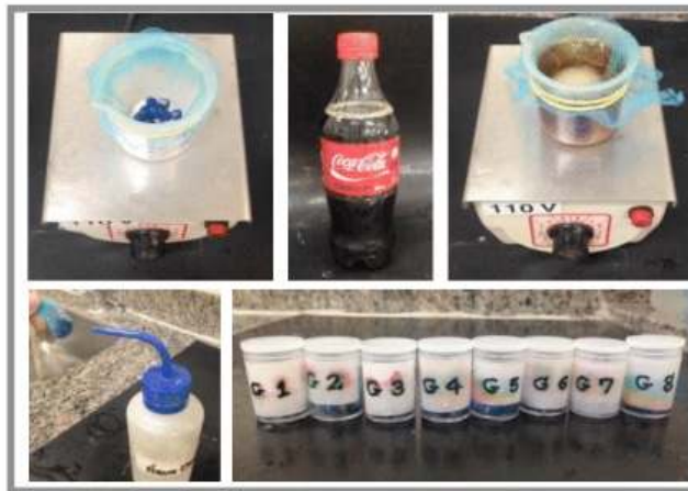
Figure 4. Realization of the erosive challenge. A) Becker with the specimens positioned on the magnetic stirrer. B) Drink used for the erosive challenge - Coca-Cola®. C) Specimens immersed in the erosive drink. D) Abundant washing of specimens with distilled water. E) Specimens stored in individualized container
