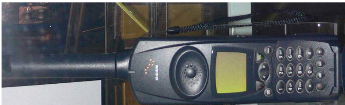
Figure 8.3.2: Motorola released the Iridium phone to the market in 1998. The phone cost $3,000 and it was literally the size of a brick. Source: http://upload.wikimedia.org/wikipedia...dium_phone.jpg .
