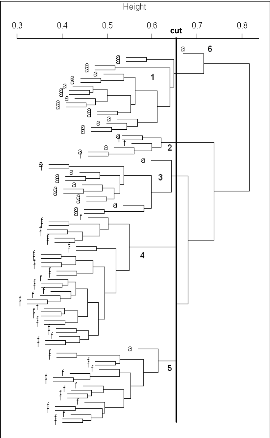
Fig. 1. Agglomerative hierarchical cluster algorithm with complete linkage. Dendrogram and clusters.
