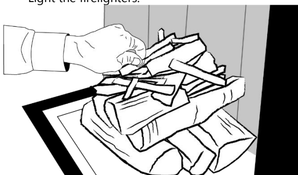
Figure 35: Lighting the fire using the "Swiss method"
