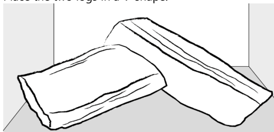
Figure 36: Position of the logs in the Kalfire W45/48F
