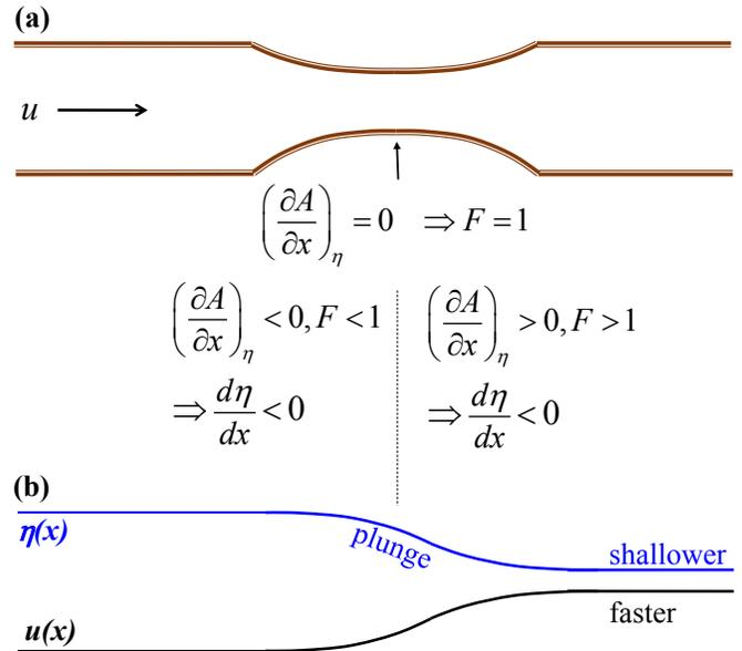
**Figure 9.6:** Flow through an arbitrary constriction. (a) Plan view. (b) Elevation and velocity profiles.
