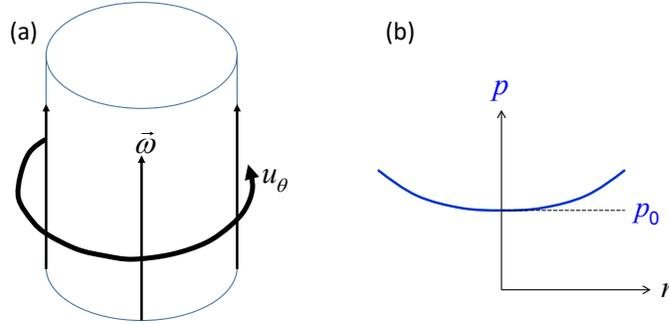
**Figure 7.7:** (a) A columnar vortex tube. (b) Radial pressure variation.
