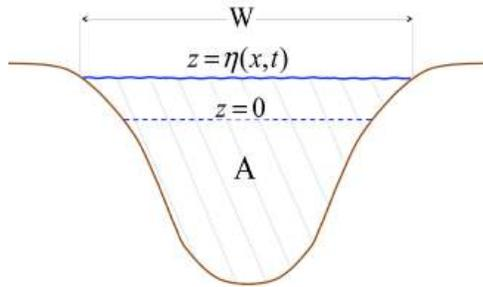
**Figure 9.5:** Cross section of a channel of arbitrary shape.  $W(x, \eta)$  is the surface width;  $A(x, \eta)$  is the wetted area.
