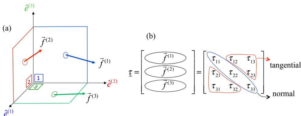
**Figure 6.5:** Stress on coordinate planes. (a) Vectors illustrate stress (force per unit area) acting on three coordinate planes. Colors indicate the force vector and the unit normal associated with each plane. (b) Array formed by the stress components,  $\tau_{ij} = f_j^{(i)}$ . Normal and tangential components are colored as in figure 6.4.
