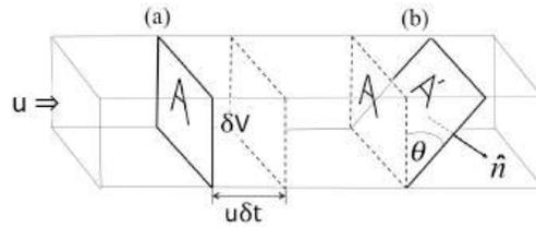
**Figure 4.2:** Volume flux through a rectangular channel. (a) A rectilinear cross-section showing the volume transport in a time  $\delta t$ . (b) A tilted cross-section with unit normal  $\hat{n}$ .
