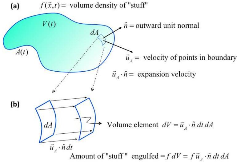
**Figure 6.1:** Definition sketch for Leibniz rule. (a) An arbitrary volume  $V(t)$  enclosed by the closed surface  $A(t)$ . (b) A small volume engulfed as the surface element  $dA$  evolves over a brief time interval  $dt$ .
