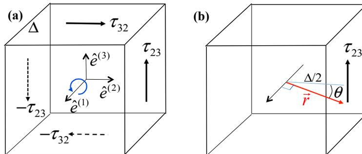
**Figure F.5:** Torques about the  $\hat{e}^{(1)}$  axis on a cube with side  $\Delta$ . (a) Tangential stresses. (b) The moment arm.
