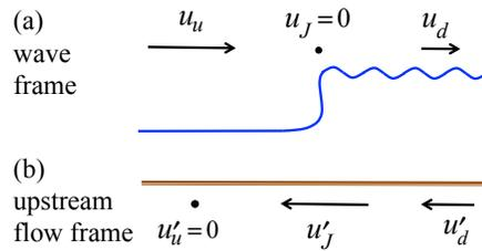
**Figure 9.11:** Definition sketch for velocities in (a) a stationary hydraulic jump (upper) and (b) a bore moving into still water (lower). The wave is the same; the only difference is the reference frame. The velocities  $u_u$  and  $u_d$  are given by (9.3.9) and (9.3.8).
