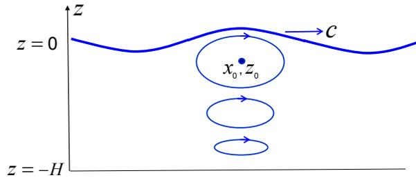
**Figure 8.4:** Elliptical particle trajectories under a small-amplitude surface wave propagating to the right with phase velocity  $c$ .
