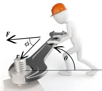
**Figure B.1:** Definition sketch for Newton's second law in rotational form. A force  $F$  is exerted at a distance  $r$  from the axis of rotation, changing the angle  $\theta$ .
