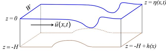
**Figure 9.2:** Two-dimensional flow in an inviscid, homogeneous fluid with a free surface. The vertical coordinate is directed opposite to gravity (upward). The mean surface is  $z = 0$  and the mean depth is  $H$ .
