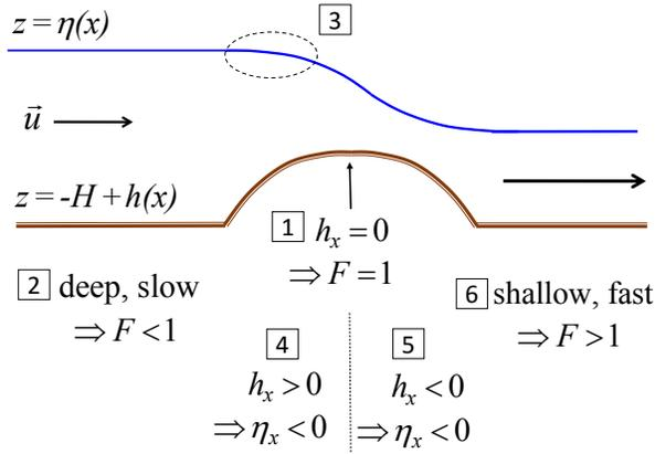
**Figure 9.4:** Steady, large-amplitude flow over an obstacle. Numerals indicate the points described in the text.
