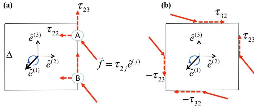
**Figure F.4:** Forces acting to rotate a cube about  $\hat{e}^{(1)}$ . (a) Effects of the same force acting at points above and below the  $x_2$ -axis. (b) Tangential forces acting on all four faces.
