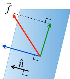
**Figure 6.4:** Stress vector at a surface, with unit normal  $\hat{n}$ , resolved into normal (blue) and tangential (green) components.
