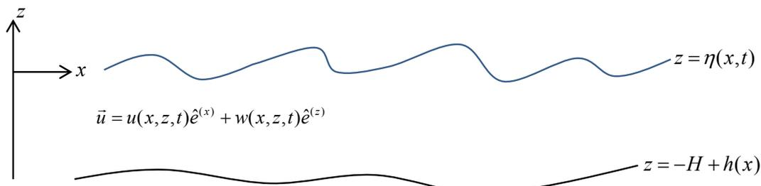
Figure 12.3: Definition sketch for two-dimensional channel flow.
