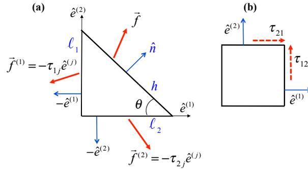
**Figure 6.6:** Two-dimensional representations of stresses acting on (a) a right triangle, (b) one corner of a rectangle. As the size of each figure goes to zero, net forces and torques must vanish.
