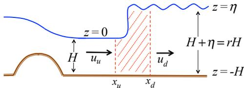
**Figure 9.8:** A hydraulic jump downstream of a constriction. The jump is enclosed by the region  $x_u < x < x_d$ . Upstream and downstream flows have velocity and depth equal to  $\{u_u, H\}$ ,  $\{u_d, rH\}$ .
