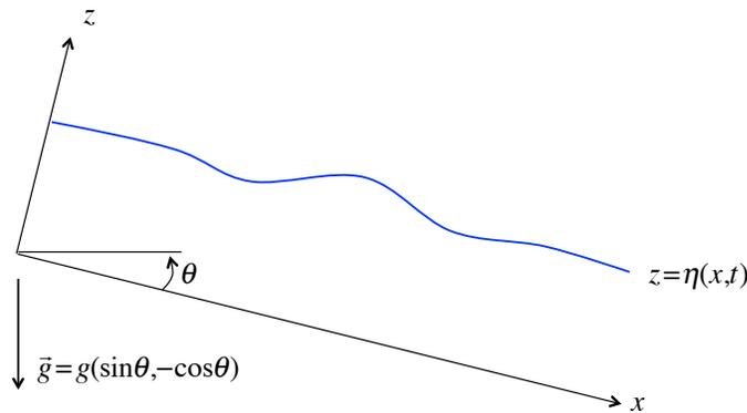
**Figure 9.12:** Definition sketch for two-dimensional, free-surface flow in a tilted channel.
