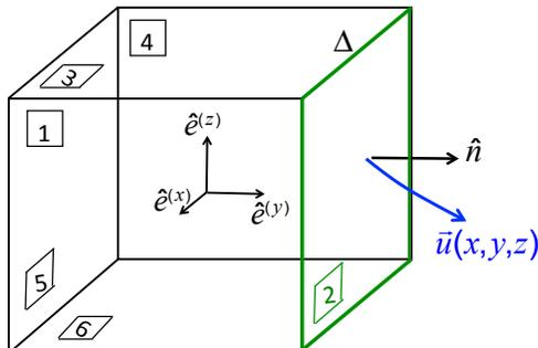
**Figure 4.4:** Definition sketch for the volume flux through a cube.
