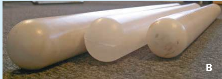
Figure 15: phase change materials (PCM) encapsulated in sealed rectangular (A) and tube (B) containers
