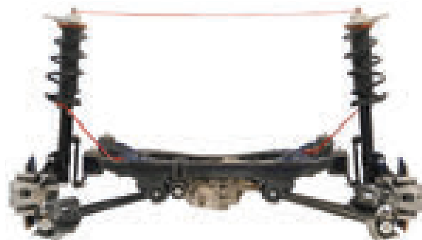
Figure 7.3.2.5 Swing half axle types
