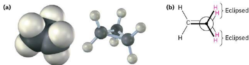
FIGURE 4.5 The structure of cyclopropane, showing the eclipsing of neighboring C–H bonds that gives rise to torsional strain. Part (b) is a Newman projection along a C–C bond.
