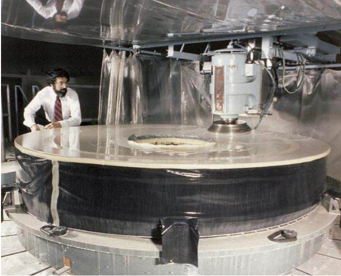
Grinding of the Hubble Space Telescope Mirror, 1979 Public Domain | Image courtesy of NASA. CC licensed content, Original
