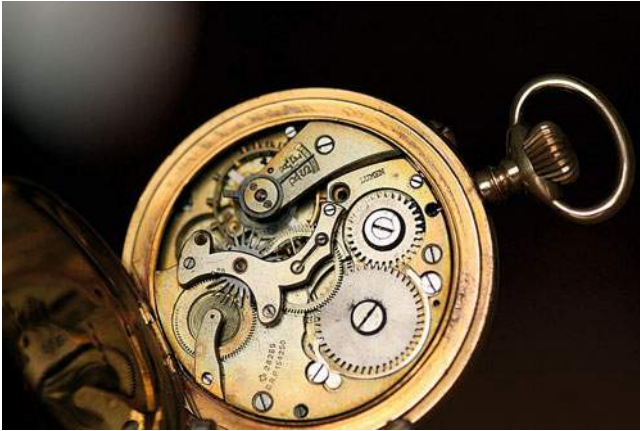
Fig. 2.32 An antique pocket watch with the English lever escapement
