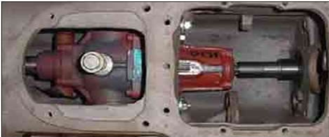
Hydrostatic transmission inside a tractor engine
